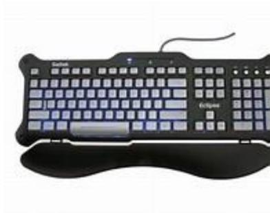
A **computer keyboard** is a typewriter-style device which uses an arrangement of buttons or keys to act as mechanical levers or electronic switches. Replacing early punched cards and paper tape technology, interaction via teleprinter-style keyboards have been the main input method for computers since the 1970s, supplemented by the computer mouse since the 1980s.
